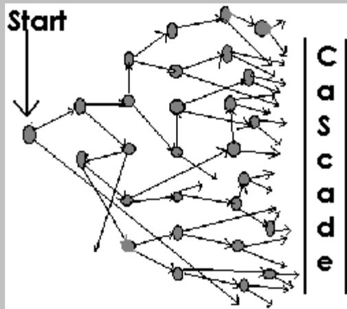
In power generation, 90 kg are not brought together, but small quantities react so that they just generate tremendous heat. And this heat is drawn off by water circulating around the fuel rods. Rods of carbon, which absorbs neutrons and knocks them out of the 'chain reaction', help control the rate of the reaction, and power is drawn from the reactor at a steady pace.
