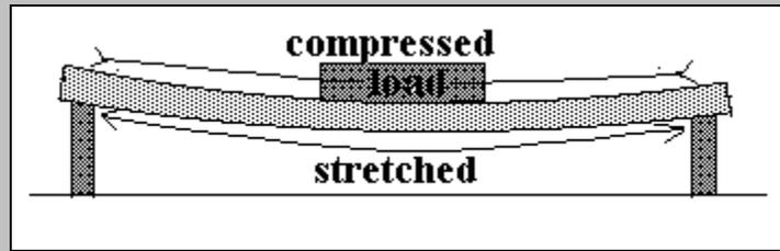
The great solution to this Achilles' heel of concrete has been to add 'reinforcement', by steel bars, to the concrete. The steel binds securely to the concrete and adds its own strength when the concrete is stretched. It may come as a surprise that steel is less elastic than concrete. The steel thus stretches less than concrete, when subjected to tension, and keeps the concrete from breaking.
