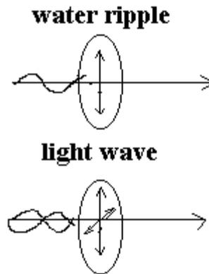
Now when light reflects or is scattered, the scattered light does not have all the planes of vibration of the original wave. In Polaroid lenses, special materials can cut out certain planes of vibration, and this generally reduces more of light that causes glare than light from illuminated objects.
