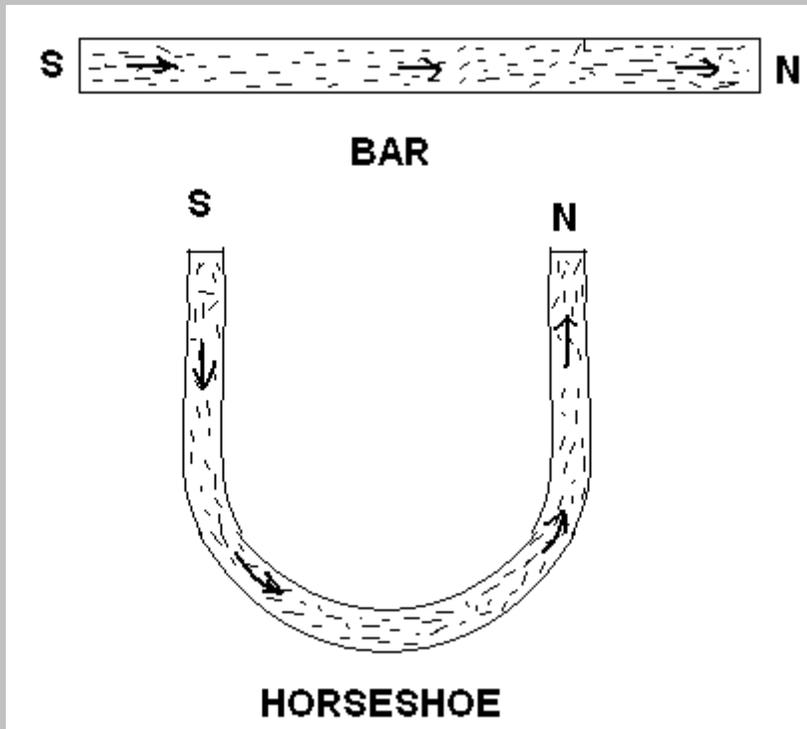
But there is a kind of magnet that has both poles on the *same side*. Mind you, this is same side, not at the *same end*. We are talking about the horseshoe magnet, which is just a bar magnet bent around like a horseshoe, with both poles pointing the same way. Horseshoe magnets create a very strong field in the cap between the poles!
