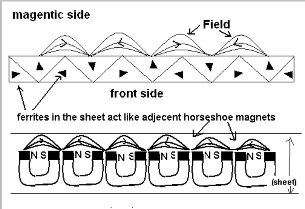
Well, that is exactly the case. Flexible magnetic sheet is made from rubber or plastic that is mixed with powdered magnetic material, usually iron-based, called ferrite. When the mixture sets, it is passed through rollers to give it the shape of a sheet and also by a matrix of strong magnets, to align the ferrites as the plastic sets. The alternate poles in the matrix orient the ferrites into little 'U's and there, the sheet is magnetic on one side but not on the other!
