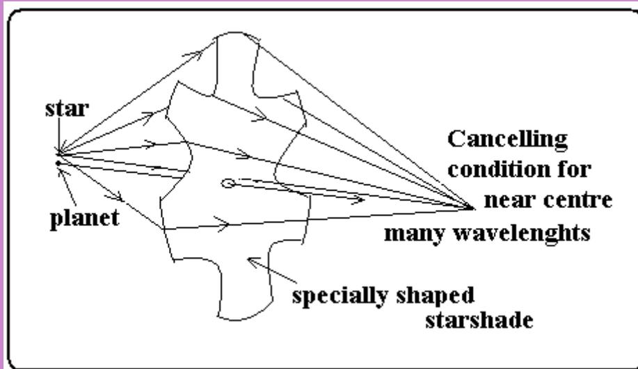
Using the mathematical theory of light in waves, Cash has developed a ‘sunflower petal-like’ shape of a starshade which is effective for a range of colours of light. A shade about 50 metres across, and managed by a spacecraft some 40,000 kms beyond an orbiting telescope, can throw a dark shadow that allows an earth sized planet around a star to be actually seen!
