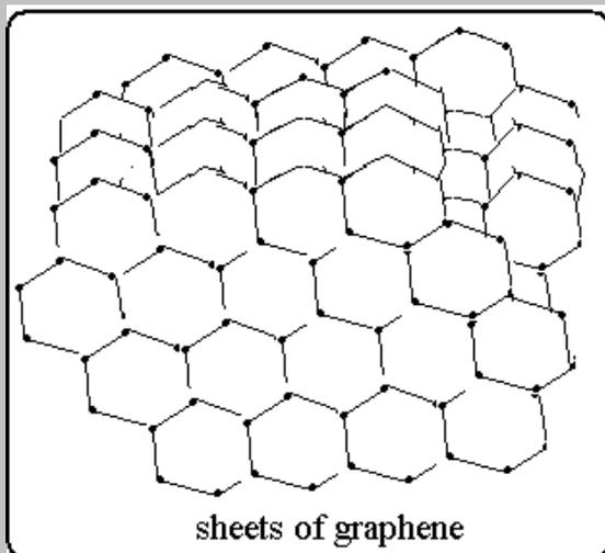
Graphene is a single layer of carbon atoms, densely packed in a honeycomb lattice. It could even be considered to be a sheet of atoms drawn out of slab of graphite. The energy distribution within the sheet of carbon atoms is a series of energy barriers for an electron trying to pass through. The various fields and spins associated with the lattice and the electrons make the behaviour follow mathematics quite akin to what PAM Dirac had devised for the electron.
