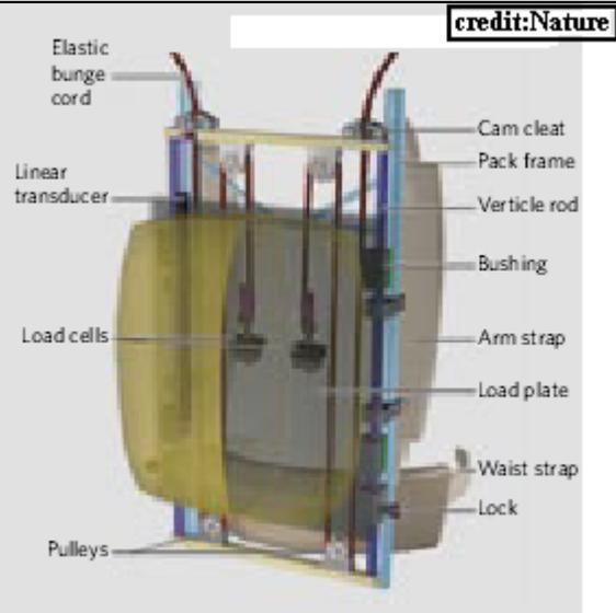
“While walking at 6.5 kmph, the vertical oscillation of a 27 kg load is reduced from 68.5 mm in the locked backpack to 26.5 mm in the suspended backpack”, says Prof. Rome in a communication published in *Nature* this week, “The metabolic cost of walking with the load falls from 640 W for the locked backpack to 600 W”, he adds.
