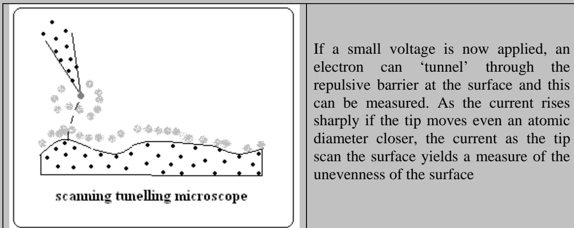
If a small voltage is now applied, an electron can 'tunnel' through the repulsive barrier at the surface and this can be measured. As the current rises sharply if the tip moves even an atomic diameter closer, the current as the tip scan the surface yields a measure of the unevenness of the surface
