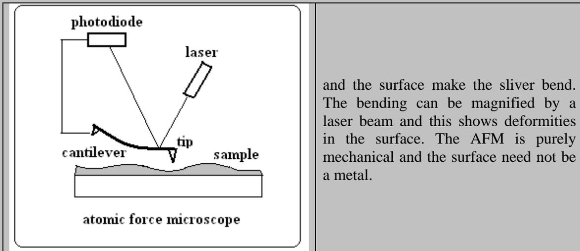
and the surface make the sliver bend. The bending can be magnified by a laser beam and this shows deformities in the surface. The AFM is purely mechanical and the surface need not be a metal.
