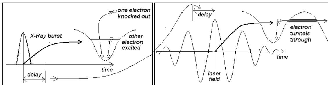
The accumulation of  $\text{Ne}^{++}$  depends on the delay between the X Ray pulse and the laser pulse – the yield increasing in steps as additional peaks in the laser pulse become available, as delay is varied. Tuning the delay indicates that excitation and tunnel ionization must occur within a total time of 300 attoseconds.
