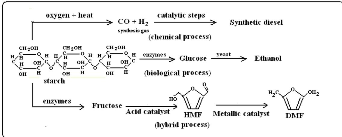
The process takes a short-cut by going from fructose directly to the final product, without coming down to carbon monoxide and building up to diesel. The other advantage is that fermentation, which is time consuming, is avoided. DMF may then become the fuel of the future.
