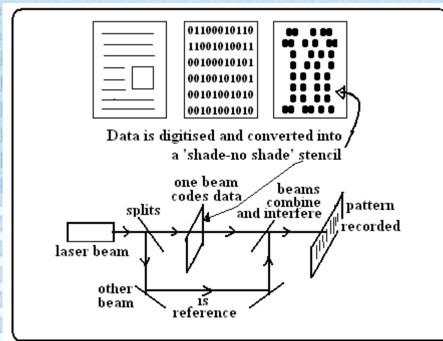
Viewing the laser source through the hologram will thus reproduce the image of the object, differently from each point of viewing, which is to say, differently for each eye and thus in three dimensions!
