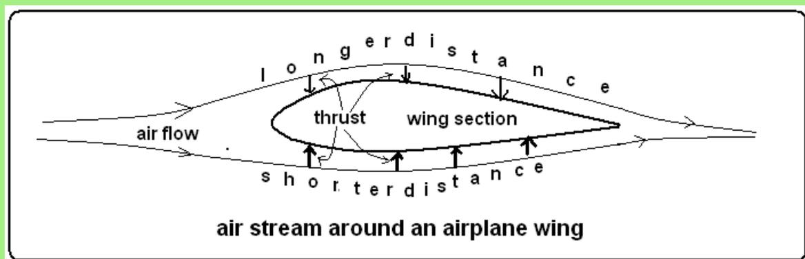
The theory is exact and simple so long as we are talking about air that moves *smoothly* around the wing. If the wing were to move very fast through the air, the relative movement would not be smooth, but would become turbulent, with whorls, eddies and uneven pressure distribution, which complicates things. The sensitive control that living things, like birds and insects, can exercise over flight seems to come from control of these complex features of fluid dynamics.
