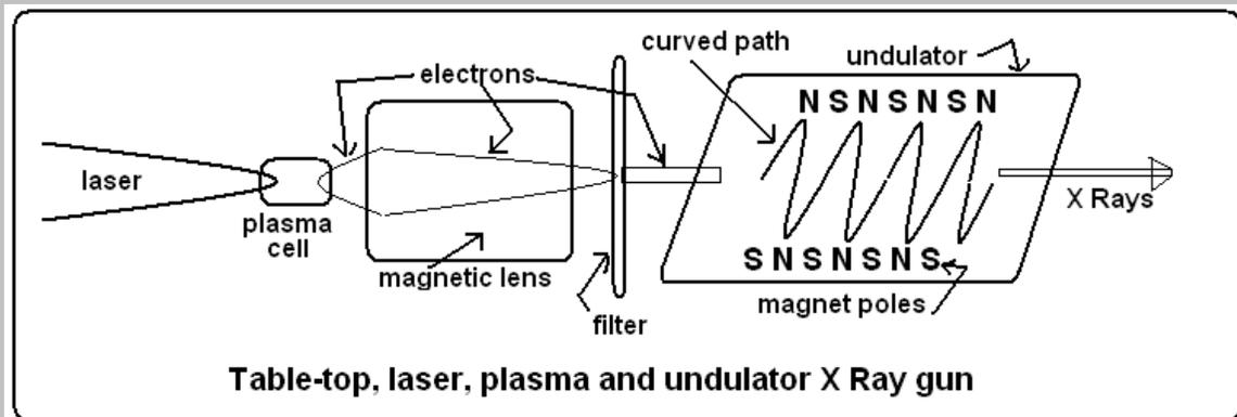
The electron beam is then passed through an ‘undulator’, a series of opposite pole magnets, just 30 cm long with magnets 5 mm apart, which twist the high speed electron beam into a rapidly curving path. The result is X Rays of the ultra short wavelengths of synchrotrons and free energy lasers, but through a table-top arrangement!
