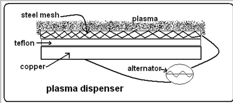
Plasma is created within the mesh, it barely warms up more than 5 degrees C, can cover comfortably the area of a pair of hands and clears bacteria down to nearly a millionth of its population in less than 10 seconds. The device generates UV radiation or toxic gases within permitted limits and is within safe limits of electrical current and voltage.
