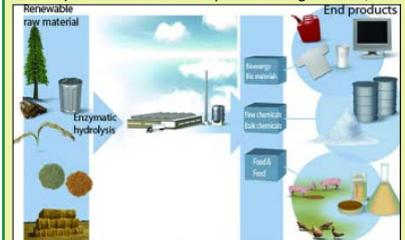
A biorefinery transforms biomass derived from renewable raw materials into a wide range of commodities by means of advanced biotechnological processes like enzymatic hydrolysis.
