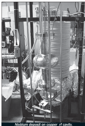
Niobium deposit on copper rf cavity.
