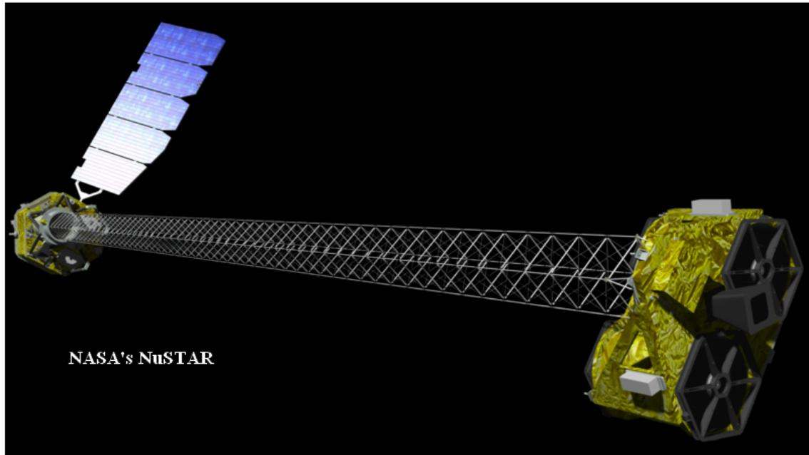
The NuSTAR optics enables detection of X Rays of about ten times the energy, or about ten times shorter wavelength than the SMM-Newton, which is a very great advance in sensitivity.
